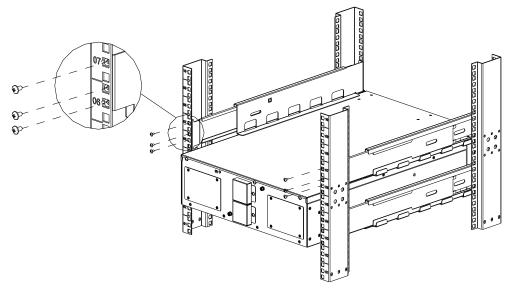
4 Secure the brackets on UPS module with 4 (M4x6) screws.
