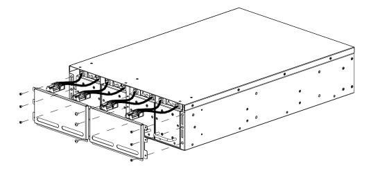
4 Remove the battery modules from the battery pack.
