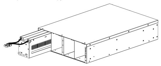
Mount the UPS and battery pack to the stabilizer bracket.
