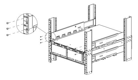
**3** Secure the back of rail with 6 (M5x12) screws.
