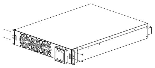
**5** Rest the UPS module on the rail shelves. Slide the UPS module into the rack.
