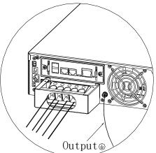
3 Connect the input wires to the first 3 terminals (counting from the left) and output wires to the last 2 terminals.
