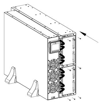
10 Install the front bezels of both the battery pack and UPS module.
