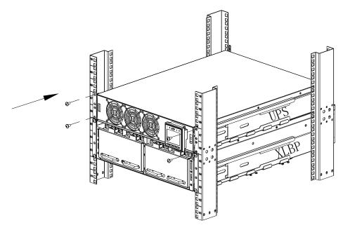
7 Install the front bezel of both the battery pack and the UPS.
