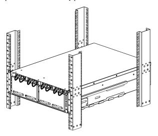
2 Secure the front of rail with 6 (M5x12) screws.
