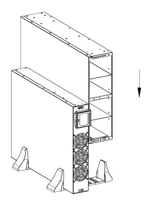
Rotate the LCD of UPS module 90 degrees to the right.
