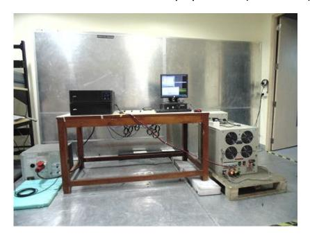
Conducted Emission Measurement: AC Input power Lines (Battery Mode)
