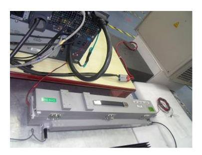
**Continuous Conducted Radio-Frequency on EPO**
