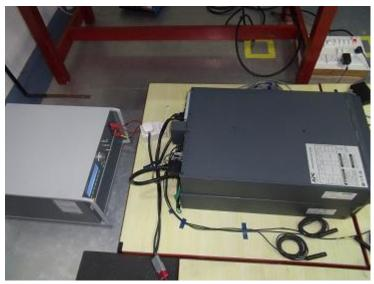
**EFT on AC input power lines**
