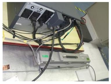
**Continuous Conducted Radio-Frequency on Ethernet on NMC**
