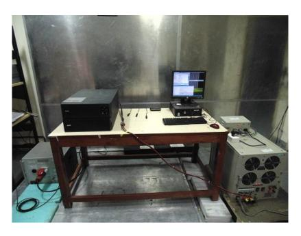
**Conducted Emission Measurement: AC Input power Lines (On Line Mode)**
