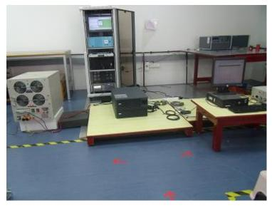
**Continuous Conducted Radio-Frequency on AC input power lines**
