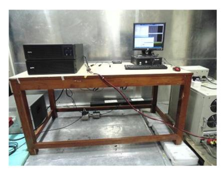
**Conducted Emission Measurement: Ethernet on Mini-rohdes**
