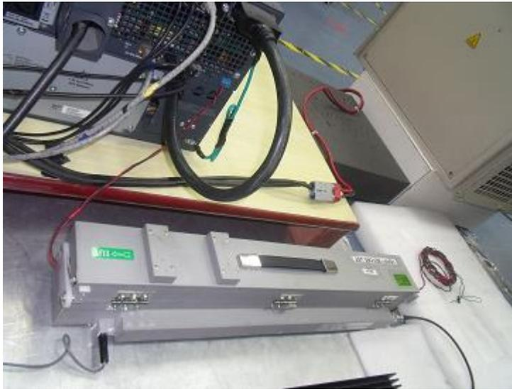
**Continuous Conducted Radio-Frequency on EPO**
