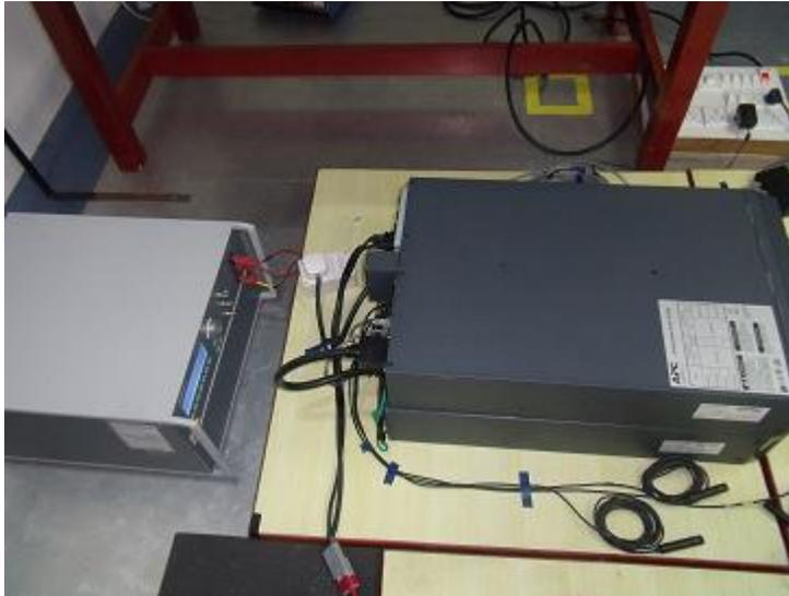
**EFT on AC input power lines**
