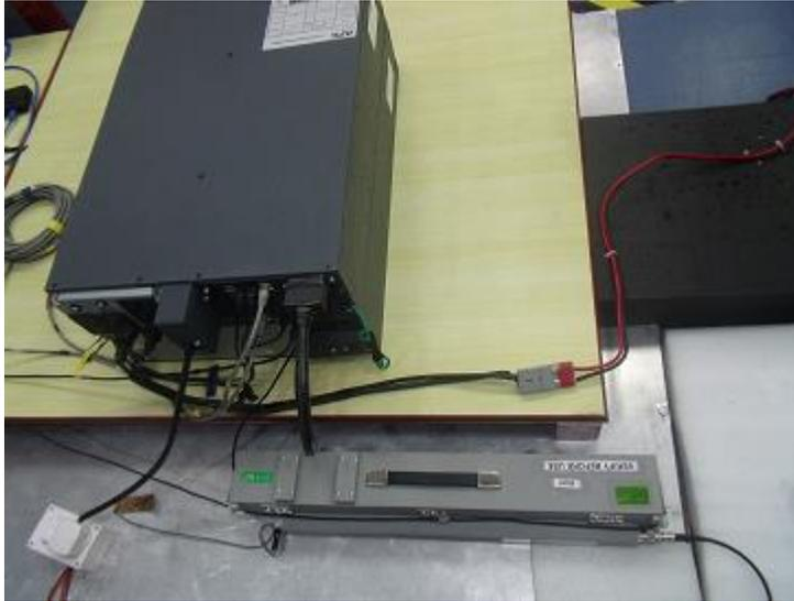
**Continuous Conducted Radio-Frequency on USB**
