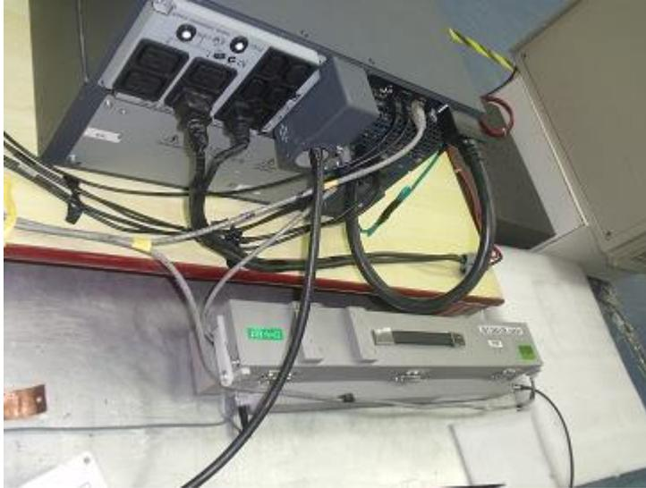
**Continuous Conducted Radio-Frequency on Ethernet on NMC**
