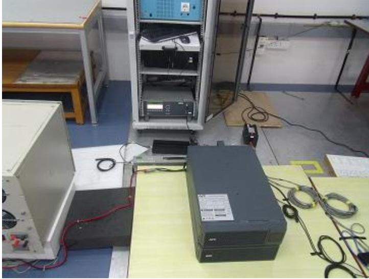
**Continuous Conducted Radio-Frequency on Universal I/O on Mini-rodhes**
