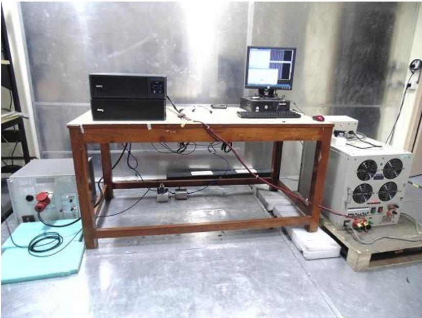
**Conducted Emission Measurement: Ethernet on NMC**
