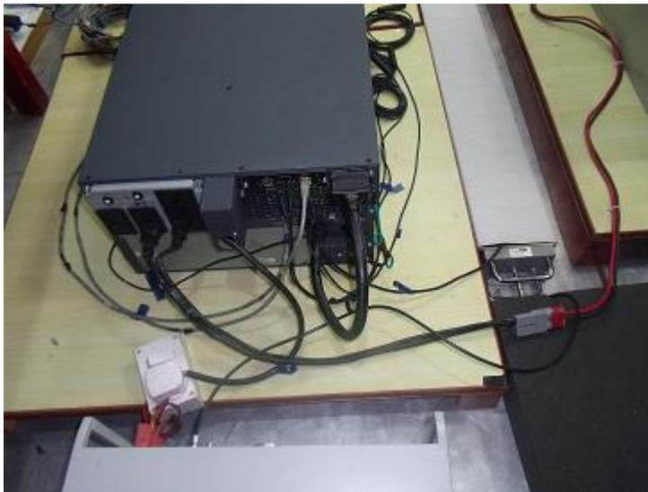
**EFT on Micro link serial communication**
