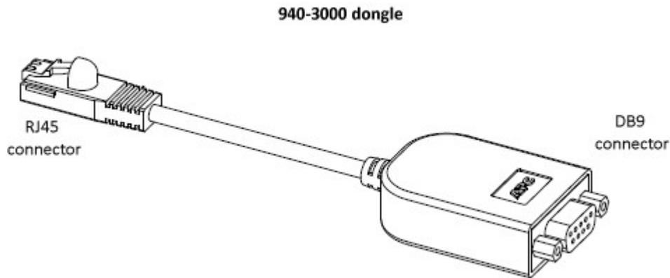
3. Choose and attach the correct **communication cable** for your system, see Which cable should you use?
