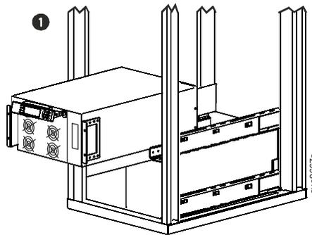
Secure the UPS and the XLBP in the rack using the cage nuts and ornamental screws included in the package.
