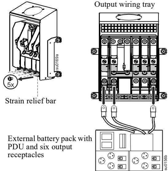
2. Connect the PDU on the external battery pack to the output wiring tray.
