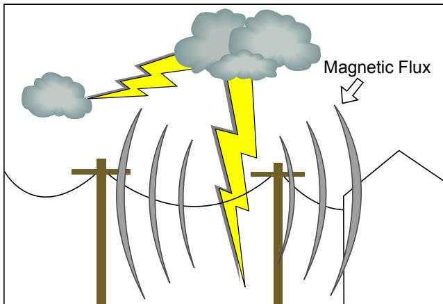
While coupling occurring between wires and from lightning strikes are two of the better-known sources of data line transients, there are other major sources of coupling that can be detrimental to data infrastructure within a facility. When planning or inspecting the layout of data lines in a facility, the following sources of inductive coupling should be addressed:
