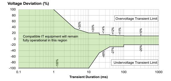
Class 2 – The output voltage has no upper bound and it is allowed to be interrupted (i.e., 0V) during the initial 1 ms of the transient. It then quickly stabilizes to within ±20% of nominal within 10 ms, and further stabilizes to within ±10% of nominal within 100 ms as shown in the green region of **Figure A6**. This level of performance is acceptable to most critical IT loads.
