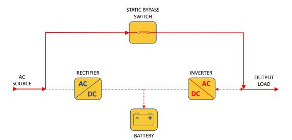
Figure 7 PFC bypass normal mode - double conversion on-line UPS topology
