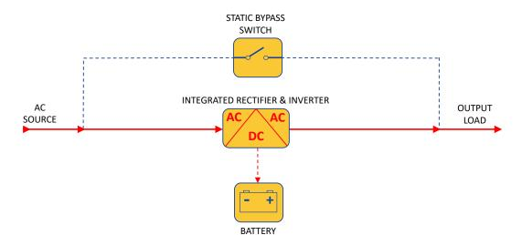
Figure 3 On-line normal mode hybrid conversion on-line I IPS tonology
