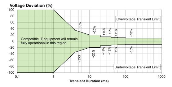
Class 1 – The output voltage is never interrupted during the transient. It stays within ±30% of nominal during the initial 5 ms, quickly comes within ±20% of nominal within 10 ms and further stabilizes to within ±10% of nominal within 100 ms as shown in the green region of Figure A7. This level of performance is acceptable to the most sensitive critical IT loads.
