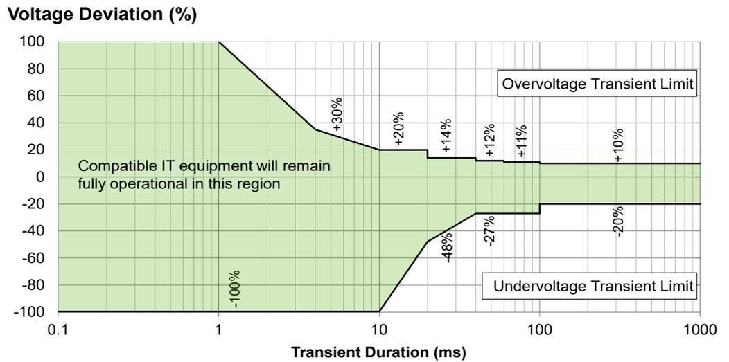
**Class 2** – The output voltage has no upper bound and it is allowed to be interrupted (i.e., 0V) during the initial 1 ms of the transient. It then quickly stabilizes to within  $\pm 20\%$  of nominal within 10 ms, and further stabilizes to within  $\pm 10\%$  of nominal within 100 ms as shown in the green region of **Figure A6**. This level of performance is acceptable to most critical IT loads.
