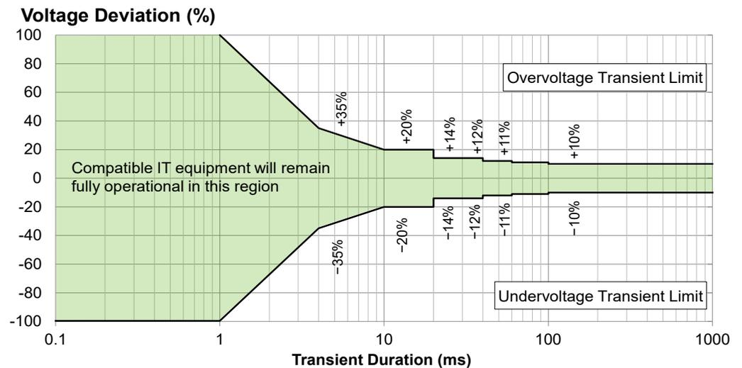
**Class 1** – The output voltage is never interrupted during the transient. It stays within  $\pm 30\%$  of nominal during the initial 5 ms, quickly comes within  $\pm 20\%$  of nominal within 10 ms and further stabilizes to within  $\pm 10\%$  of nominal within 100 ms as shown in the green region of **Figure A7**. This level of performance is acceptable to the most sensitive critical IT loads.
