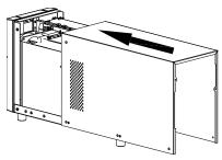
10. Fix the screws (10 nos.) securing the top cover. Please cross check the number of screws.
