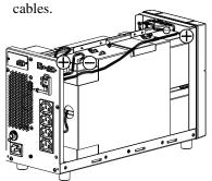
8. Fix the screws (5 nos.) securing the battery plate.
