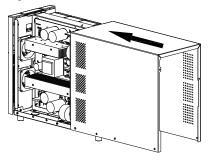
8. Fix the screws (8 nos.) securing the top cover.
