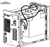
5. Remove the battery plate and the old batteries.
