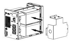
7. Make series connections as original one. Connect batteries again to PCB. Put back the battery plate.
