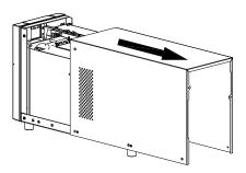
4. Locate the screws (10 nos.) securing the battery plate and unfasten them. Please cross check the number of screws.
