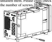
5. Remove the battery plate and the
