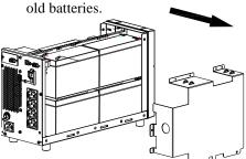
7. Make series connections as original one. Connect batteries again to PCB. Put back the battery plate.
