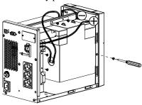
10. Fix the screws (8 nos.) securing the top cover.
