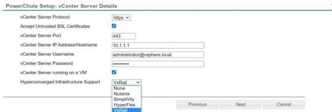
The screenshot shows the 'PowerChute Setup: vCenter Server Details' window. The 'Hyperconverged Infrastructure Support' dropdown menu is open, displaying a list of options: VxRail, None, Nutanix, SimpliVity, HyperFlex, and VxRail. The 'Next' button is highlighted in blue.
