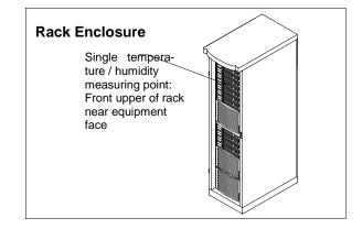
Use a temperature-humidity probe that interfaces with currently used operating and control systems to monitor and provide proactive warning of out-of-range humidity conditions (Figure 2). Many hand-held monitoring devices available allow for spot-checking of temperature and relative humidity anywhere in the room.
