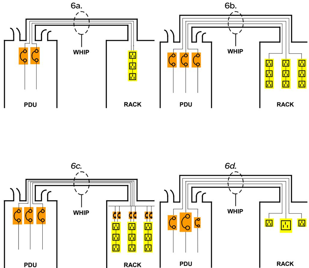
The analysis of this paper suggests that distribution whips that include single or 3-phase 30 A whips are not preferred except in the case of dedicated whips. The 30 A whip value isn't optimal because the most common branch circuit size that must be generated in a rack is 20 A, which leads to two undesirable problems with a 30 A whip size:
