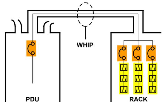
The arrangements of **Figure 5b** and **5c** are capable of providing the same power, but with a different wiring and circuit breaker arrangement. Note that in **Figure 5b**, the conduit or “whip”<sup>4</sup> contains multiple branch circuits. These alternatives give rise to significant advantages and disadvantages as summarized in **Table 2**.
