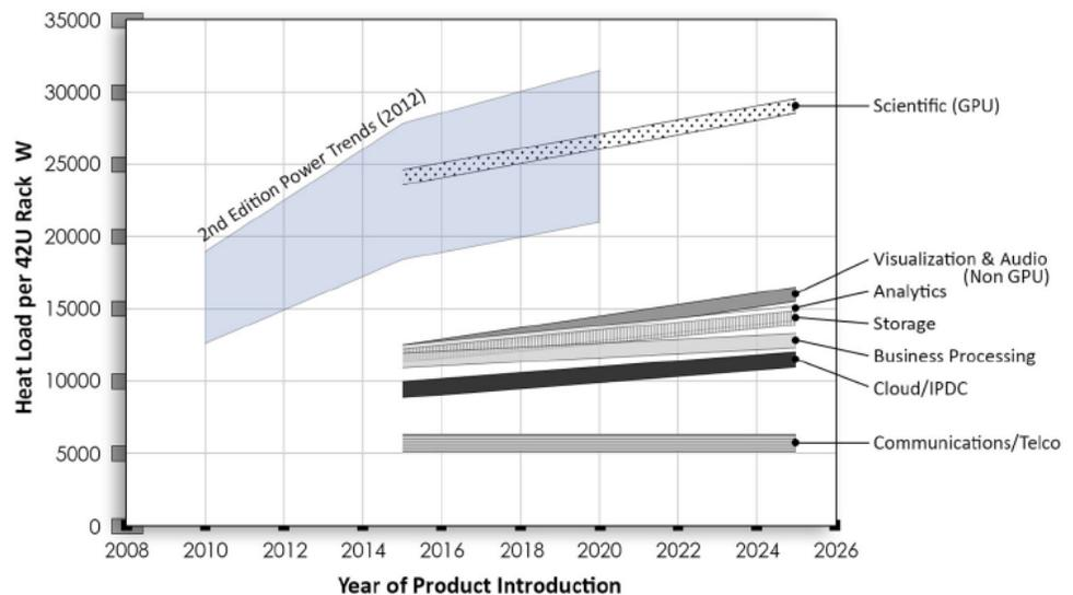
**Figure 3** shows the expected rack power density range (typical and maximum) with business processing and scientific workloads. The expected rack density with business processing workloads could range from 9kW to 22kW while the expected rack density with scientific loads could range from 23kW to 55kW.
