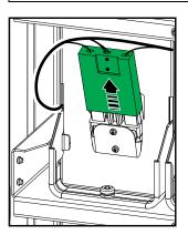
9. Remove the battery modules from the two upper rows. Leave the battery modules in the two bottom rows to increase weight stability.
