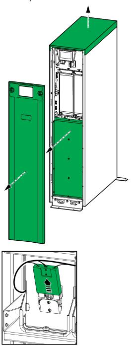
4. Remove the rear gland plates and the rear brush plates from the UPS. These are for signal cable routing.
