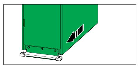
4. Lower the front and rear leveling feet on the UPS with a wrench until they connect with the floor. Use a bubble-leveler to check that the UPS is level.
