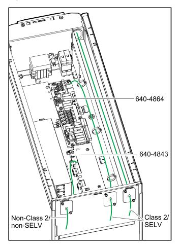
15. Reinstall all removed plates and covers. See Final Installation, page 53 for details.
