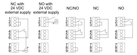
The EPO input supports 24 VDC.
