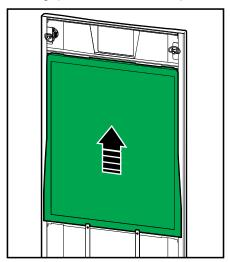
3. Hold the new air filter by the sides and insert the air filter by pushing it upwards into the door frame until you can ease it in over the two metal grips.
