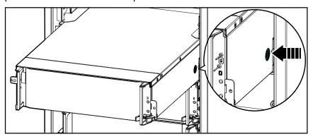
d. **Only on scalable UPS models**: If no replacement power module will be installed: Install a filler plate in front of the empty power module slot.
