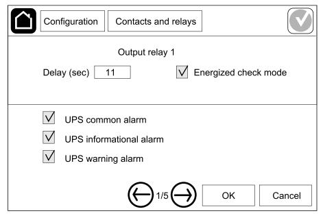
**NOTE:** It is possible to assign several functions to the same output relay.
