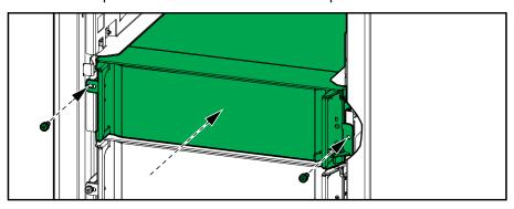
The power module will perform a self-test, automatically reconfigure according to the system, and then go online.
