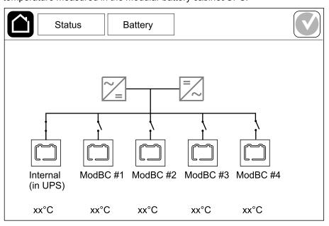
2. Tap the battery symbol named **Internal (in UPS)** (only present for UPS models for internal batteries) to see the information for modular batteries in the UPS or tap the battery symbol named **ModBC** # x to see the information for modular battery cabinet x. You will then be able to see details for each battery string such as number of installed battery modules, alarm presence, temperature for each battery string, and battery module type.
