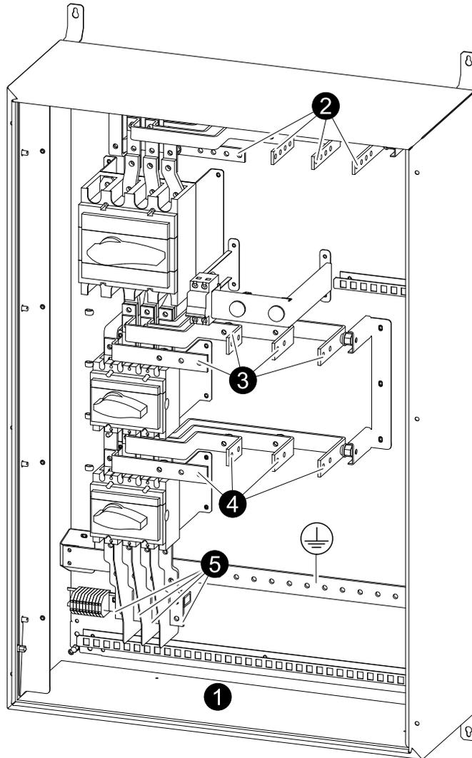
1. Route the cables through the holes in the bottom plate of the maintenance bypass enclosure.
