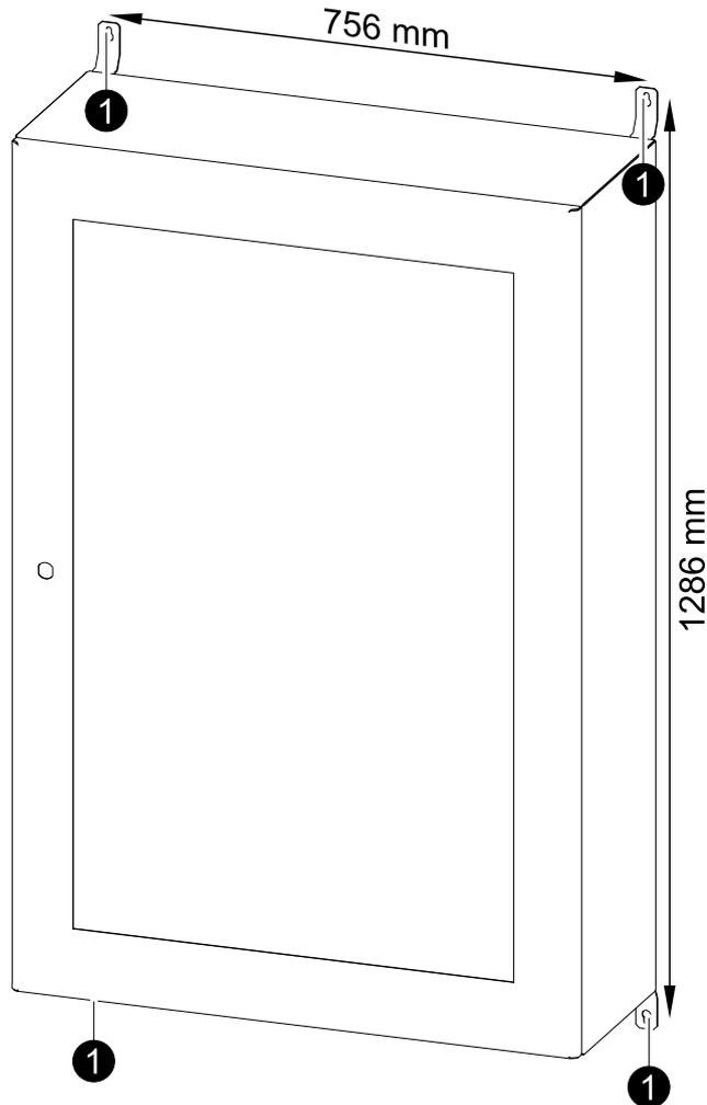
2. Drill holes in each of the four marked locations and mount the anchor bolts.
