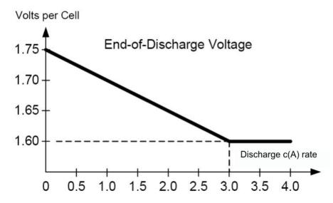
**NOTE:** C equals I<sub>discharge</sub> divided by the battery Ah capacity.
