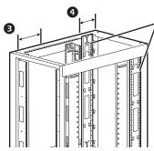
**NOTE:** Move or remove the vertical 0U Accessory Channel for rear of cabinet installation.
