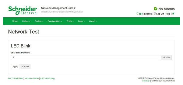
If you are having trouble finding your unit, enter a number of minutes in the LED Blink Duration field, and then click Apply. The Status LED on the Ethernet port will blink for the specified number of minutes. (The Ethernet port is on the user connection plate; see the *Operation Manual* on www.APC.com).
