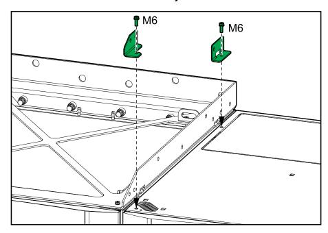
5. Fasten the top anchoring bracket to the seismic kit part with the provided M8 screws.
