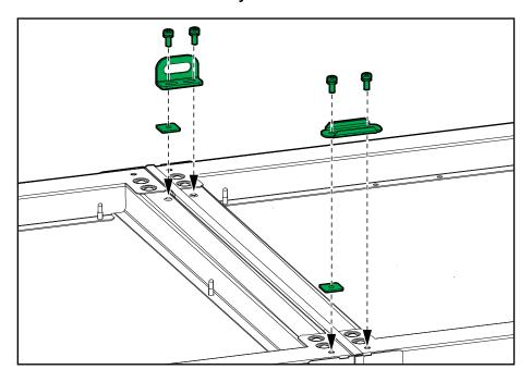
2. Mount the three M6 screws from the installation kit in the three marked positions from the power cabinet side to tighten the two cabinets together.
