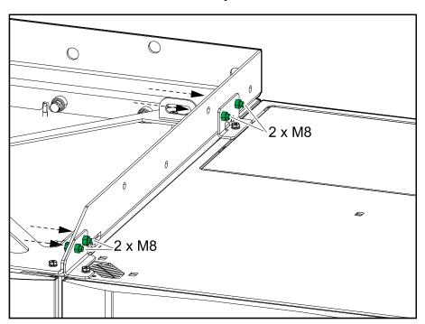
6. In systems with more than one modular battery cabinet, assemble the seismic kit parts with the provided M8 bolts and nuts.
