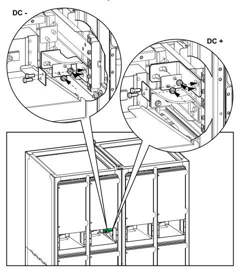
9. Reinstall the protection covers in the right side of each modular battery cabinets. Leave the cover off the modular battery cabinet that will be connected to the power cabinet.
