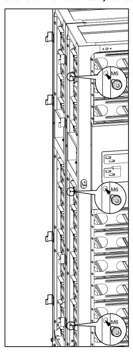
3. Remove the battery cover in the bottom right corner of each modular battery cabinet.
