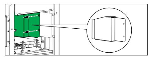
8. Install the DC + and DC – busbar assemblies between all modular battery cabinets.
