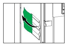
3. Remove the isolation cover from the sides of the modular battery cabinets that will be placed up against another cabinet.
