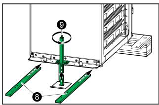
Lower the cabinet down onto the support using the jack and the drilling machine.
