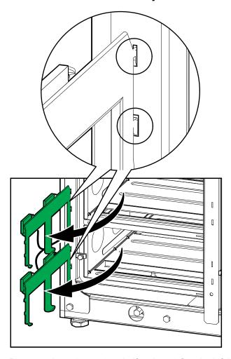
4. Place two batteries on the shelf and push first the left battery and then the right battery into the cabinet.
