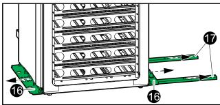
Modular Battery Cabinets Mechanical Assembly
