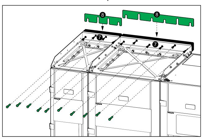
8. Place the provided plates over the M12 bolts between the seismic kit parts and the wall to fill up the gap between the wall and the modular battery cabinets.
