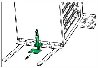
11. Place the floor protection plate under the pallet on the front of the cabinet.
