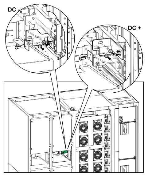
5. Reinstall the protection cover in the right side of the rightmost modular battery cabinet.
