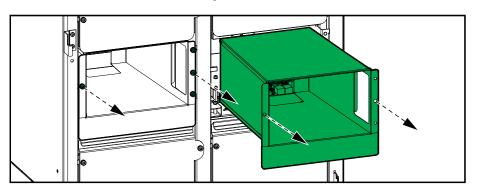
7. Remove the protection cover in the right side of each modular battery cabinet.
