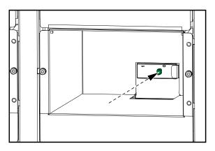
2. Loosen the bolts and remove the battery securing brackets.
