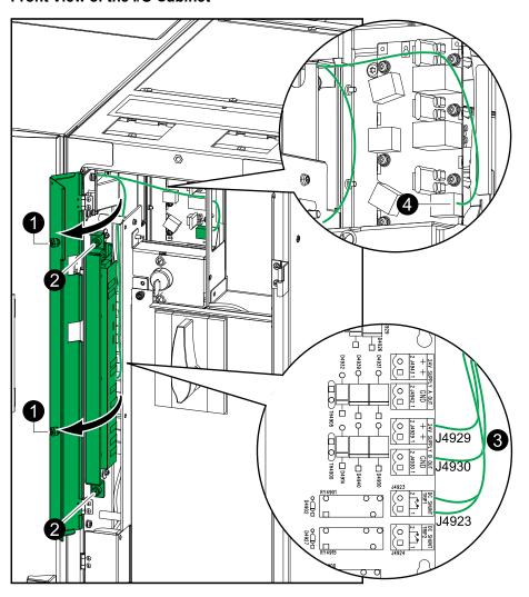
5. Route the signal cables 0W11394 and 0W11395 as shown on the illustration to the rightmost modular battery cabinet.
