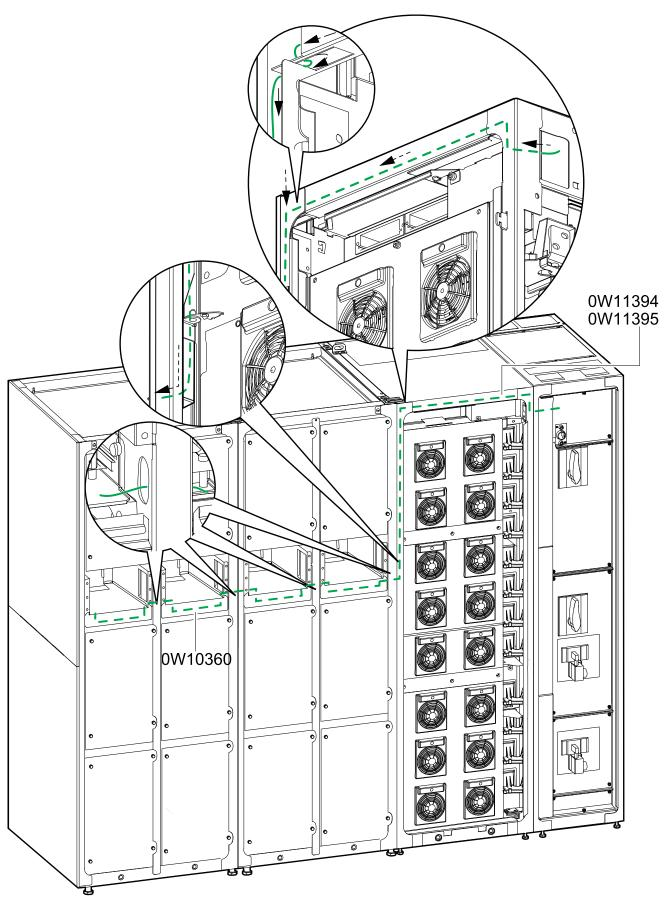
6. Connect the ABUS cable 0W11394 to the J2002 terminal in the rightmost modular battery cabinet.
