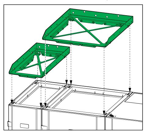
2. Fasten the seismic kit parts to the top of the modular battery cabinets with the provided M6 screws.
