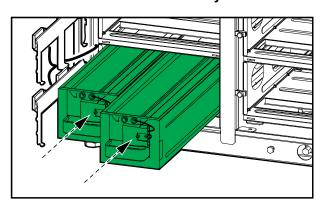
5. Reinstall the battery securing brackets by first pushing them into the holes in the right frame and then in the shelf.
