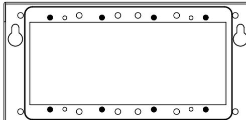
1. Install a junction box or a switch box behind the wall. The EPO box will fasten directly to the box. Use one of the options above.
