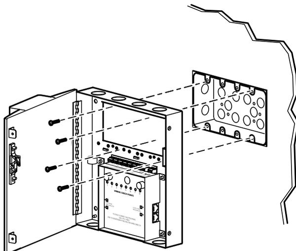
7. Reinforce the EPO box with 6 mm (1/4 in) screws in the corner mounting holes.
