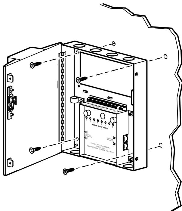
3. Install an appropriate fitting with a lock-nut for each knockout used.
