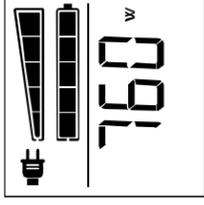
Pressing the Display/Hold to Mute button a *fifth time* displays the ONLINE output voltage (V), in this example 230 V is displayed.
