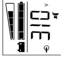
When you press the Display/Hold to Mute button a *fifth time* the ON BATT input load in Watts (W) is displayed, in this example 760 W is displayed.
