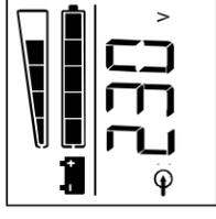
When you press the Display/Hold to Mute button a *sixth time* the ONLINE output frequency (Hz) is displayed.
