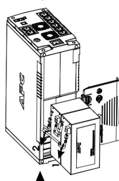
INSTALL NEW BATTERY & RECONNECT THE WIRES.
