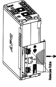
DISCONNECT BATTERY WIRES.
