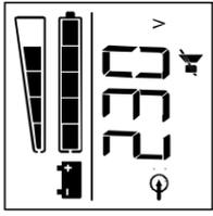
When you press the Display/Hold to Mute button a *fourth time* the ON BATT input voltage is displayed.
