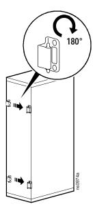
4. Remove the screws securing the hinges in the door. Reposition and reinstall the hinges.
