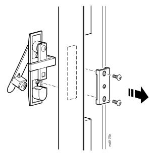
6. Remove the screw, latch, and washer from the door handle assembly. Rotate the washer 90 degrees and the latch 180 degrees; then reinstall the washer, latch, and screw.
