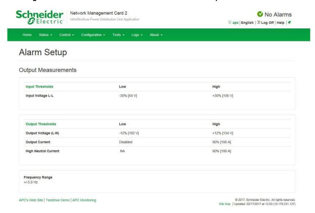
For each measurement, a value below the **Low** threshold or above the **High** threshold generates an alarm. Select **Input Thresholds** or **Output Thresholds** to configure alarms:
