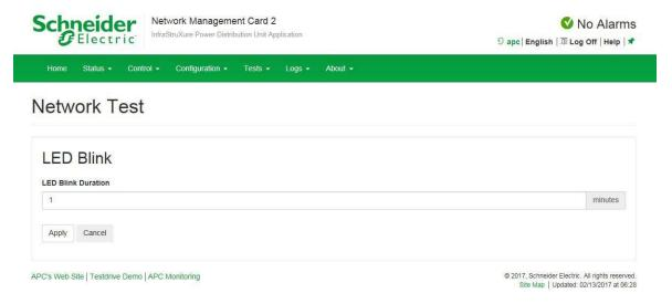
If you are having trouble finding your unit, enter a number of minutes in the **LED Blink Duration** field, and then click **Apply**. The Status LED on the Ethernet port will blink for the specified number of minutes. (The Ethernet port is on the user connection plate; see the *Operation Manual* on **www.APC.com**).
