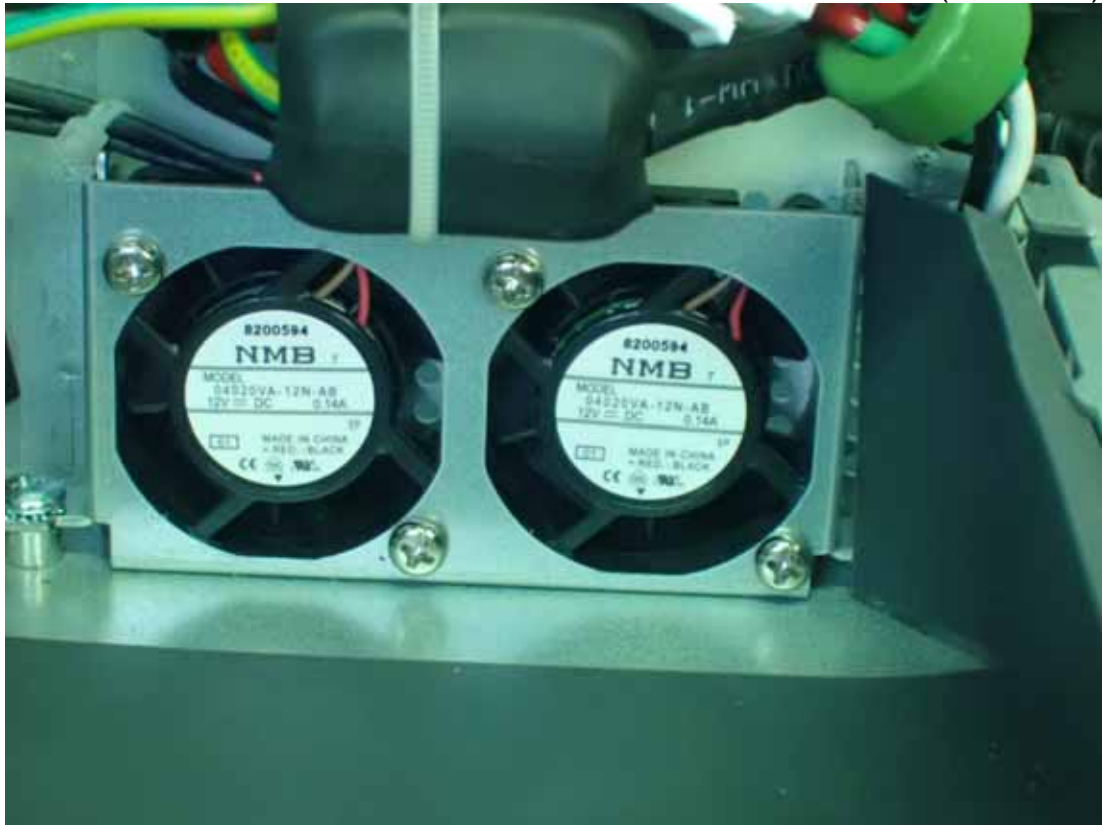
Figure 19 Internal View (FAN View)
