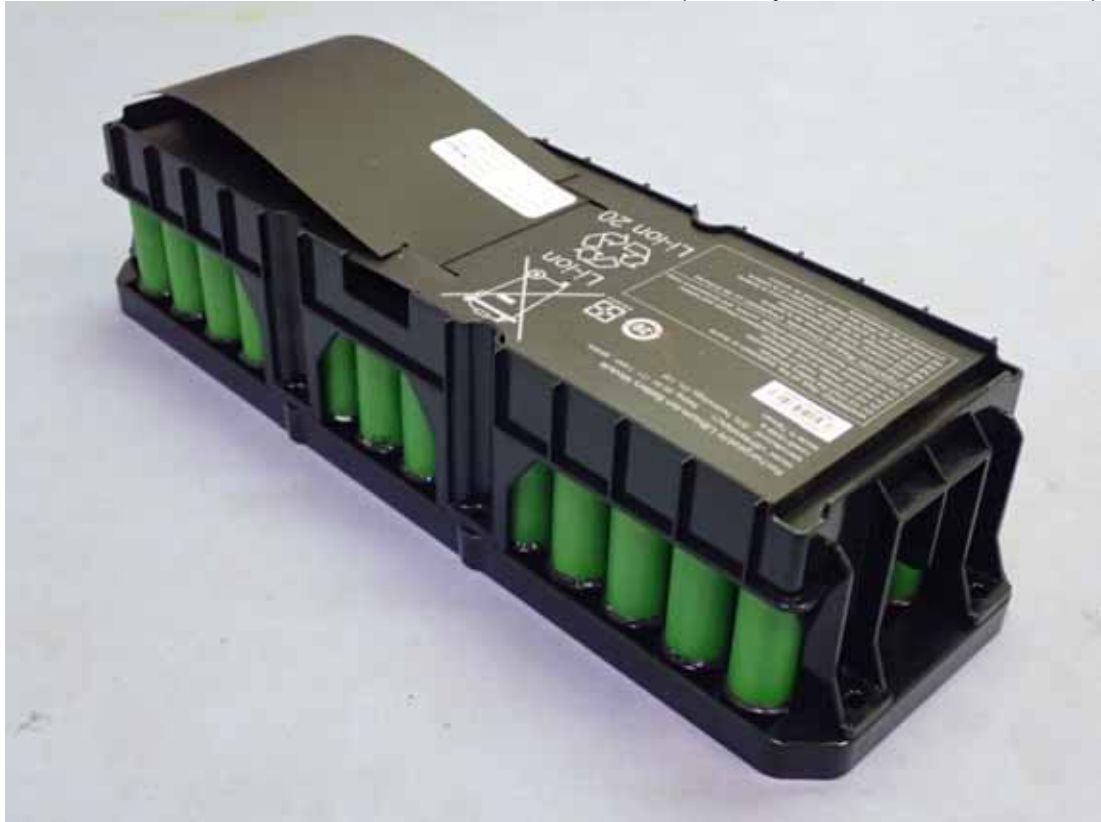
Figure 9 Internal View (Battery, Front & Side View)
