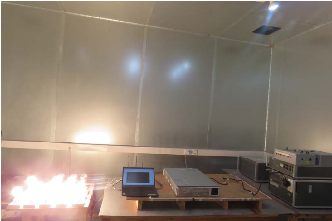
Picture 6 Surge & Dips Test Setup
