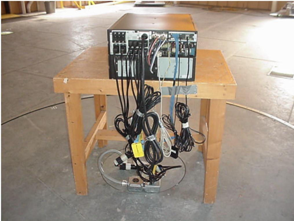
**Configuration for Radiated Emissions (Rear)**
