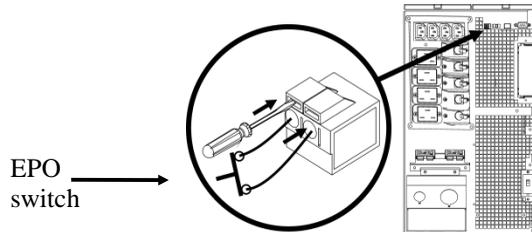
Both Class 2 and SELV circuits must be isolated from all primary circuitry. Do not connect any circuit to the EPO terminal block unless it can be confirmed that the circuit is Class 2 or SELV. If circuit standard cannot be confirmed, use a contact closure switch.
