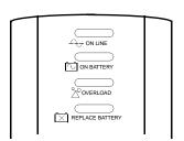
$\triangle_{+}$  On Line (green) - is lit whenever utility power is powering the Battery Backup
