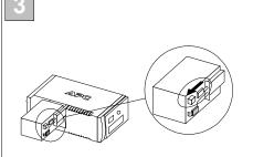
Slide the new battery into the battery compartment. Connect the battery wires to the terminals as follows: Black wire to Ground (-) terminal
