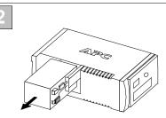
Pull the battery out, exposing the battery terminals and wires. Disconnect the wires from the terminals
