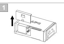
Place the unit on its side. Slide the battery compartment cover upward and off of the UPS.
