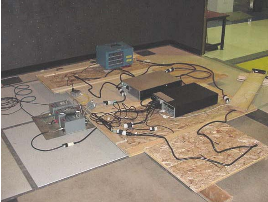
EUT Setup for EN61000-4-6 on Mains
