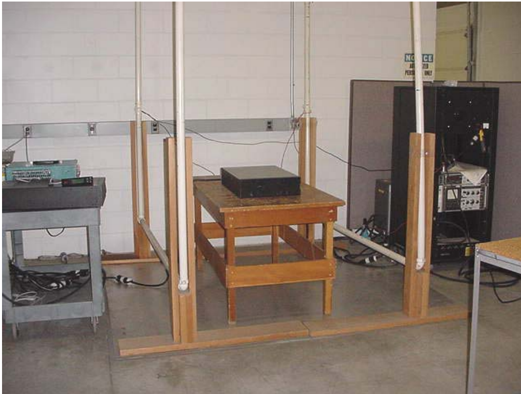
EUT Setup for EN61000-4-8
