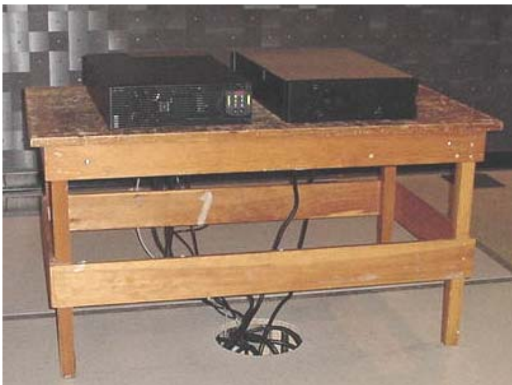
EUT Setup for EN61000-4-3 (0°)
