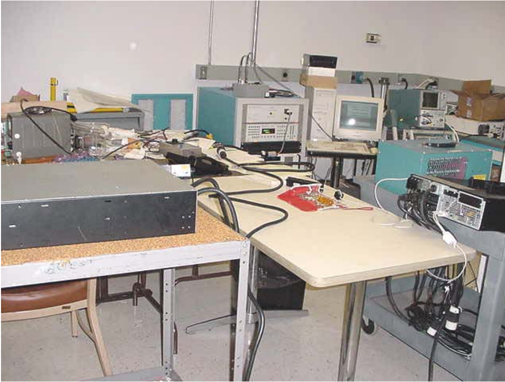
EUT Setup for EN61000-4-11
