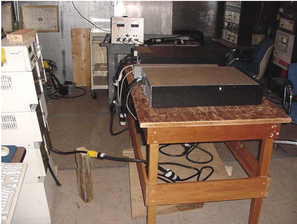
EUT Setup for EN61000-4-4 and -5 on Mains
