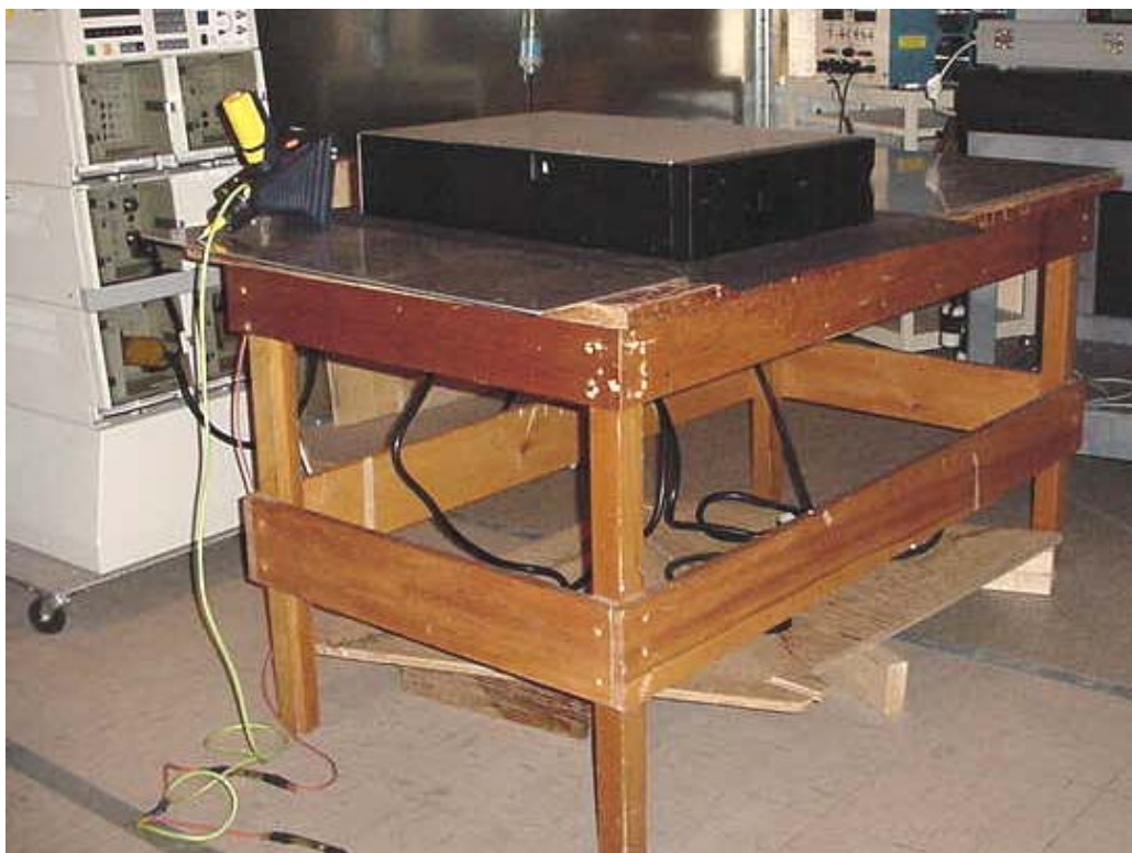
EUT Setup for EN61000-4-2
