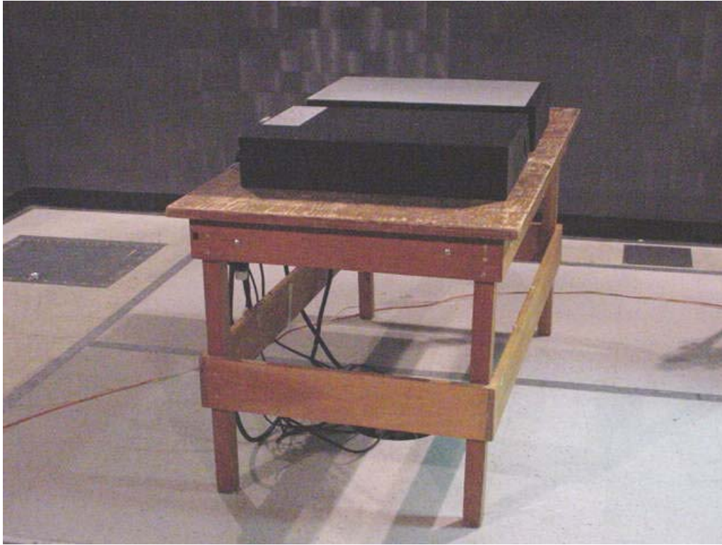
EUT Setup for EN61000-4-3 (270°)
