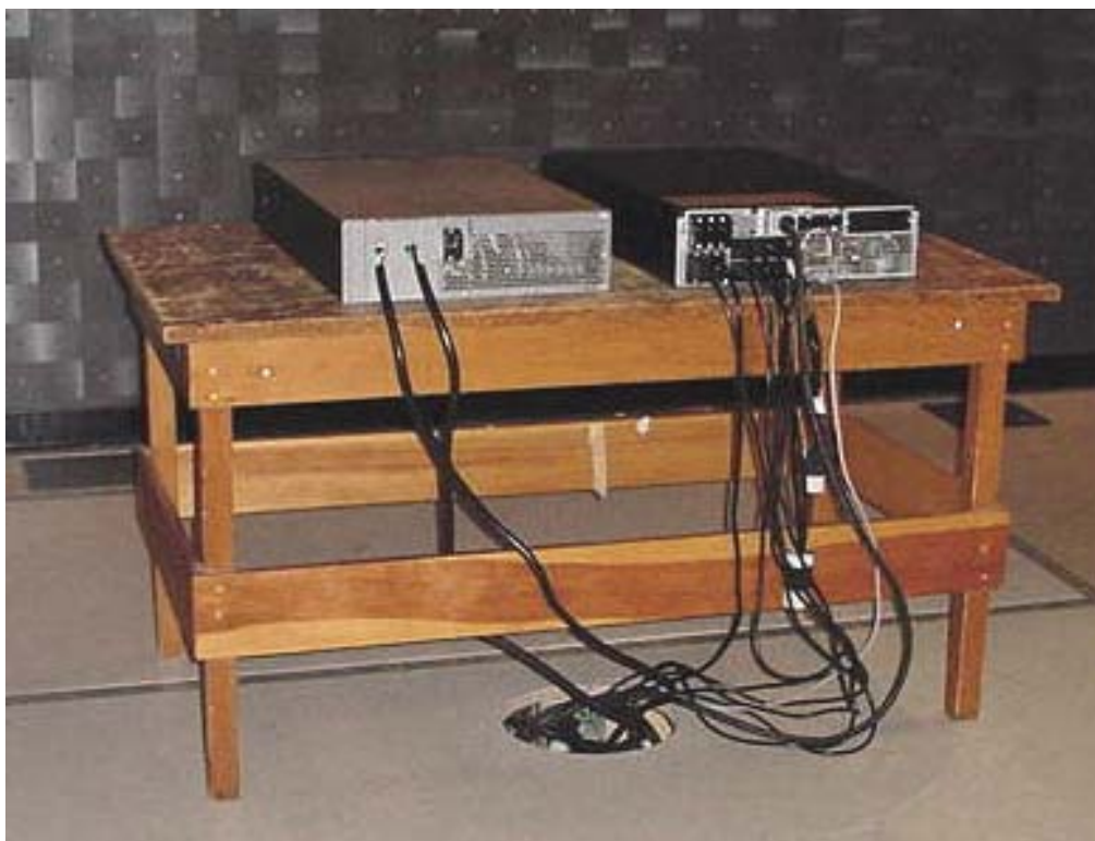
EUT Setup for EN61000-4-3 (180°)
