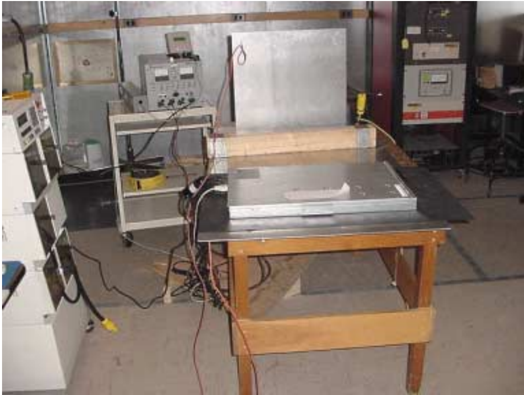
EUT Setup for EN61000-4-2
