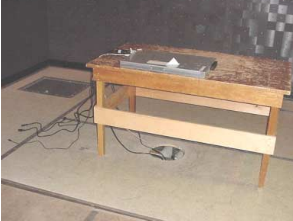
EUT Setup for EN61000-4-3 (270°)
