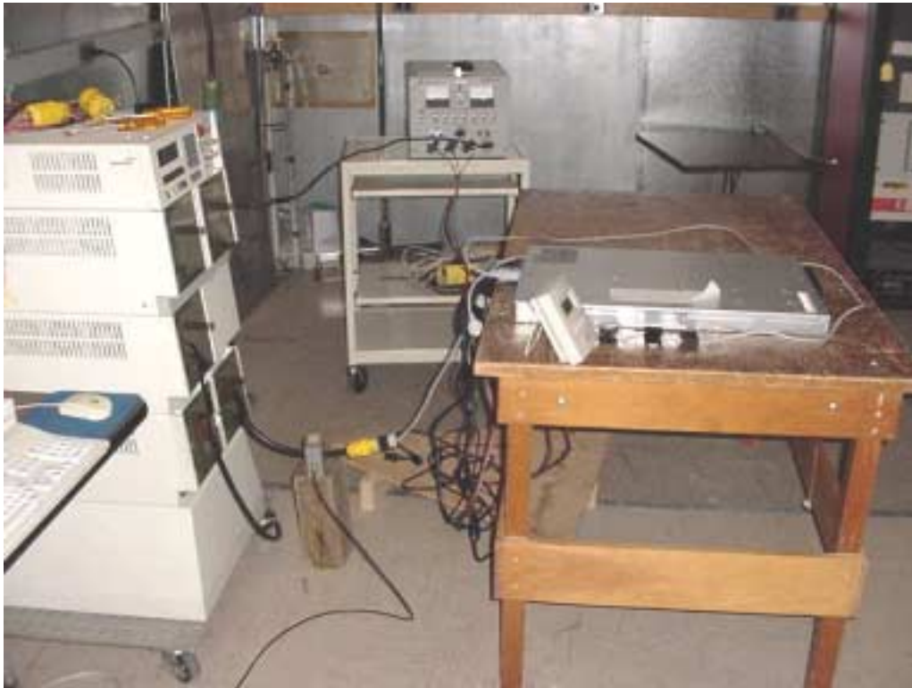
EUT Setup for EN61000-4-4 on Mains
