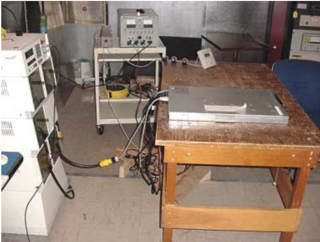
EUT Setup for EN61000-4-5 on Mains
