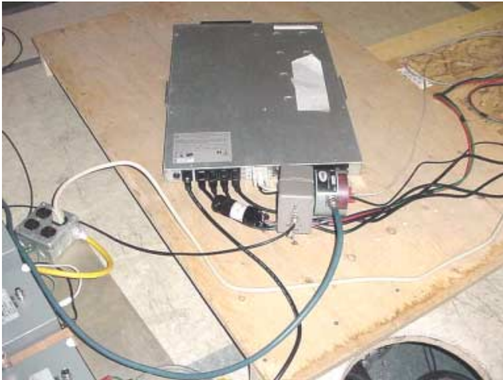
EUT Setup for EN61000-4-6 on Data Cables
