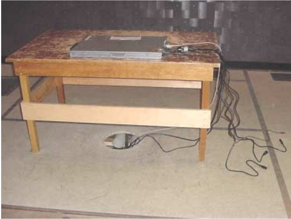
EUT Setup for EN61000-4-3 (90°)
