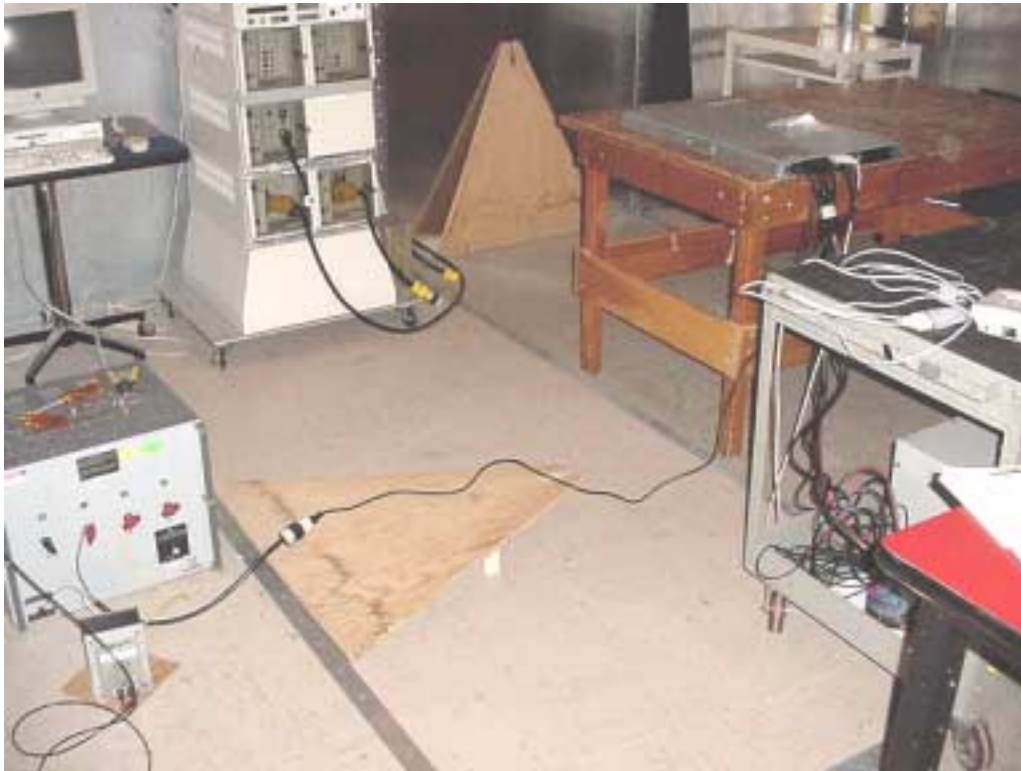
EUT Setup for IEC 1000-2-2
