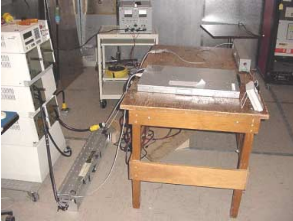
EUT Setup for EN61000-4-4 on Data Cables
