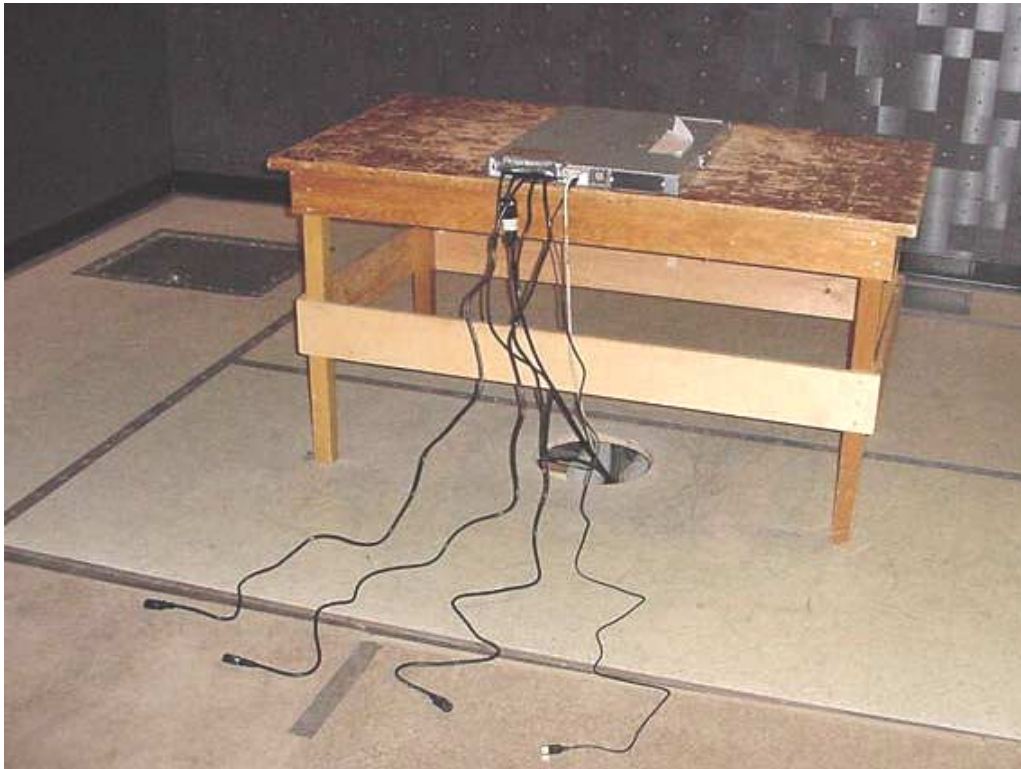
EUT Setup for EN61000-4-3 (180°)
