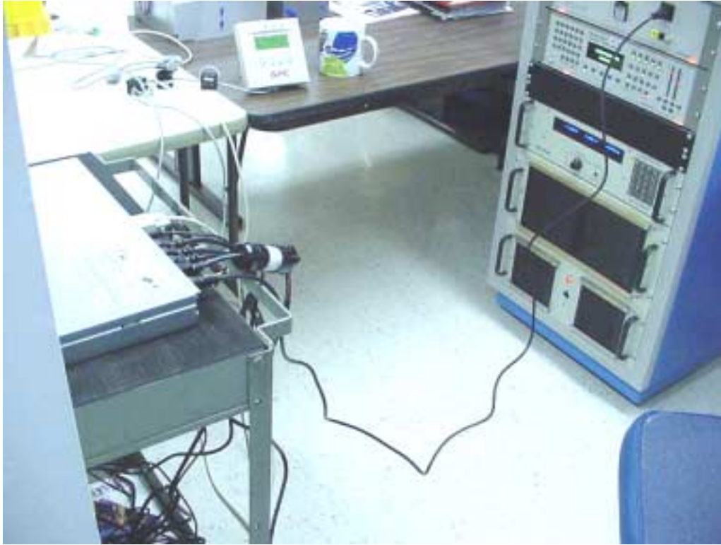
EUT Setup for EN61000-4-11
