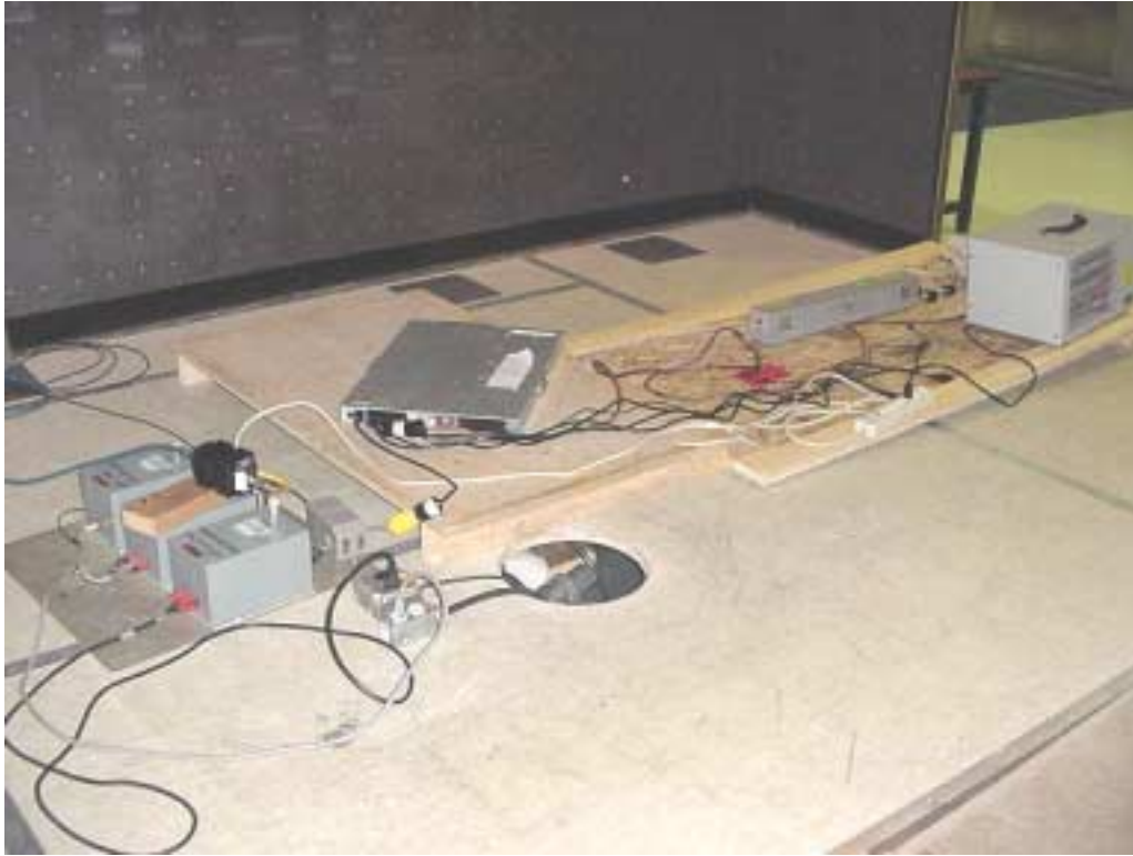
EUT Setup for EN61000-4-6 on Mains
