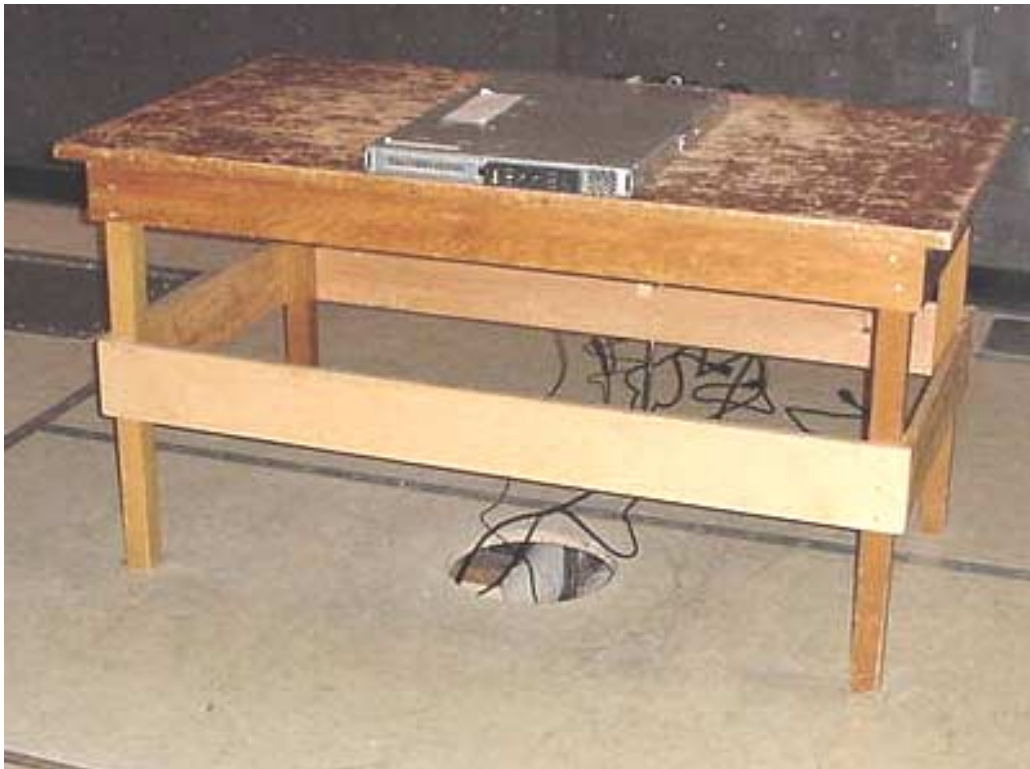
EUT Setup for EN61000-4-3 (0°)
