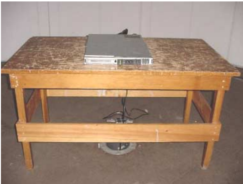
Configuration for Radiated Emissions (Front)
