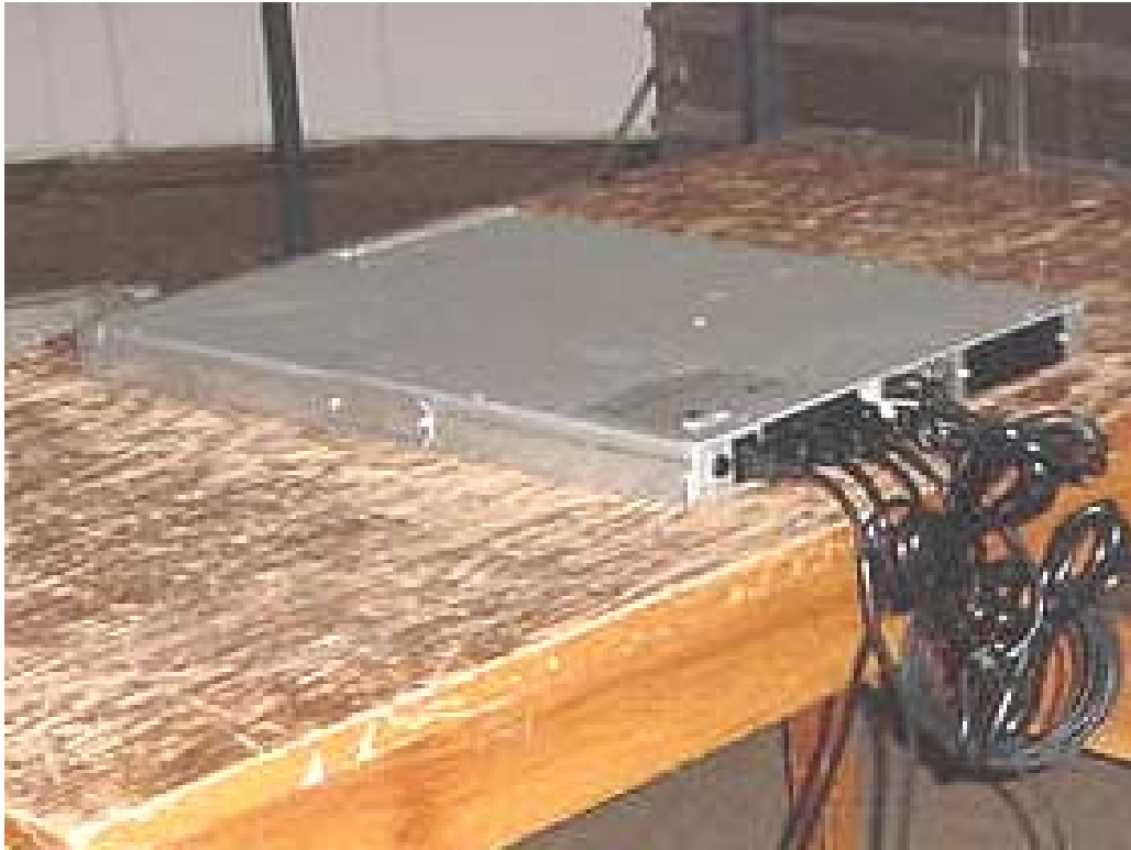
Configuration for Radiated Emissions (Rear Closeup)
