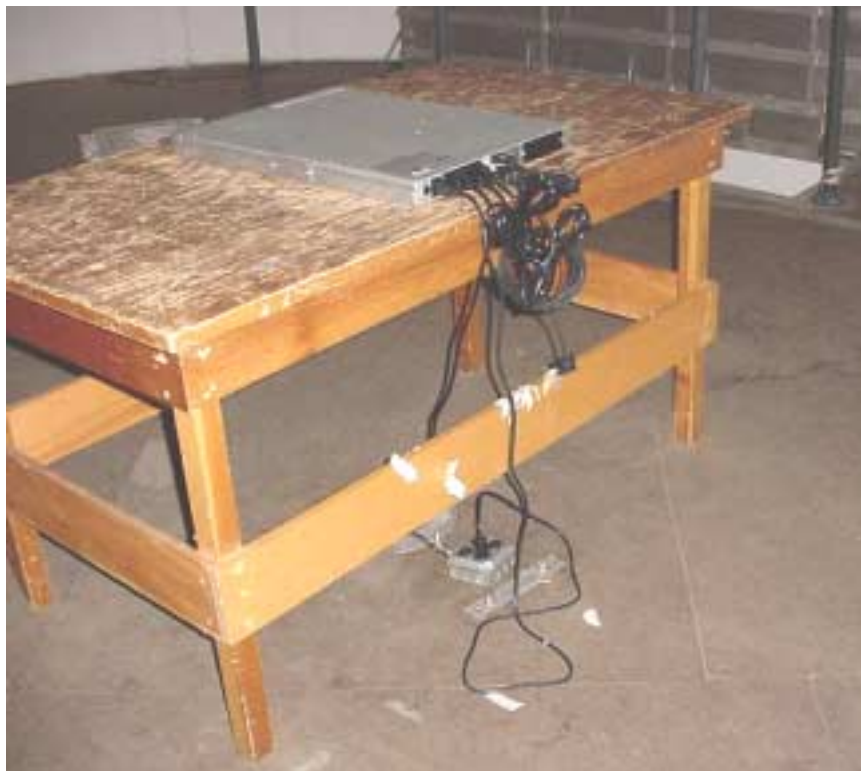
Configuration for Radiated Emissions (Rear)
