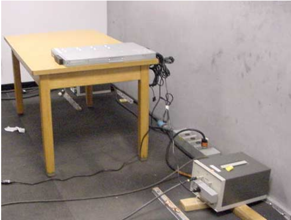
Configuration for Conducted Emissions
