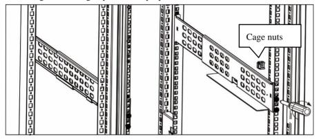
4. Put UPS on the rail support and fix the UPS in position with screws.
