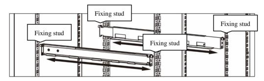
2. Use 4 pieces of M6 screws to mount rail sliders into chassis. See below chart.
