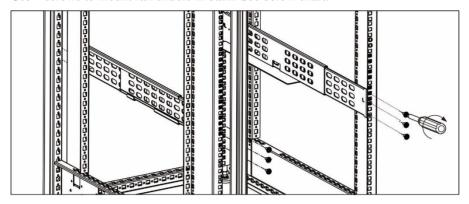
3. According to UPS height, put nuts on proper location.
