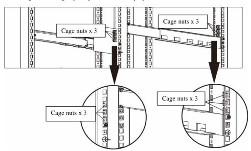
4. Put UPS with assembled ears on the rail support.
