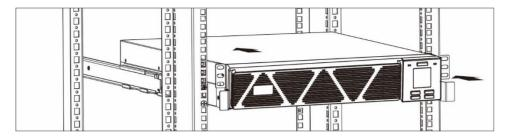
5. Fix the UPS in position with 4 screws.
