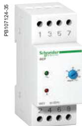
iRCP Phase control ■ Monitors the order and asymmetry of phases and the presence of voltage on the 3 phases of a three-phase circuit (power supply of a motor, etc.)
