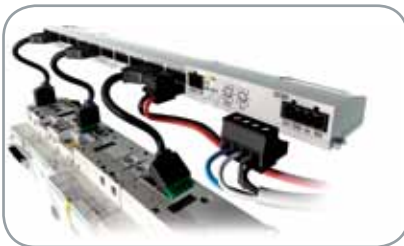
Reflex easily connects to Modbus network through Acti 9 Smartlink
