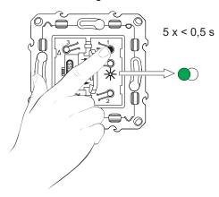
3. Remove the knob and short press the push button 5 times in quick succession.
