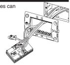
Modules should be clipped into grids before screwing product to the wall.
