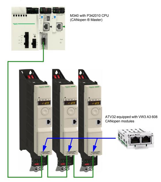
This chapter describes how to integrate an ATV32 in a unity project and to control it from a M340 PLC. Example of configuration:
