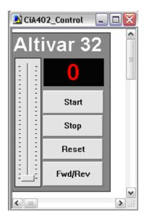
The objects of the animation screen are used as input and output parameters of the control Block. The Block is called cyclically in a SR part of the Mast task. The variables used as parameters in the following control block call are used in the previous animated table.
