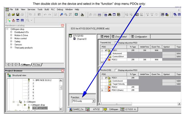
In the example above, we select only TPDO1 and RPDO1 which provides the basic control command of the drive with the CiA402 velocity mode profile.
