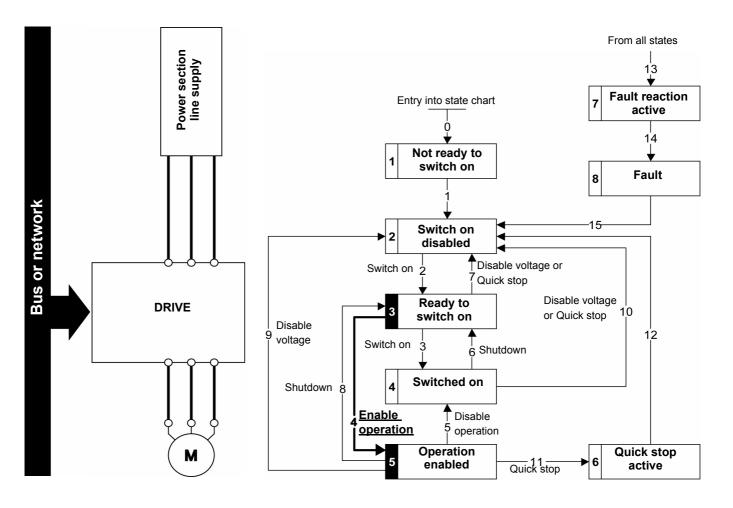
**NOTE**: It is possible, but not necessary, to send the "3 - Switch on" command followed by the "4 - Enable Operation" command to switch successively into the states "3 - Ready to Switch on", "4 - Switched on" and then "5 - Operation Enabled".
