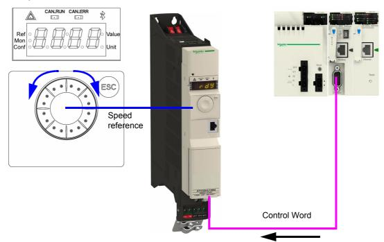
The drive is controlled from the communication (1 of the 3 following settings MDB, CAN or NET) but the reference is adjusted on the HMI. The control word comes from the controller and is written according to CiA402 profile.
