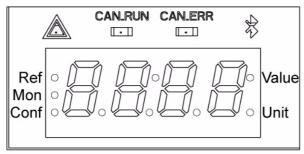
CANopen activity LEDs (CAN ERR and CAN RUN) are located on the HMI of the ATV32:.
