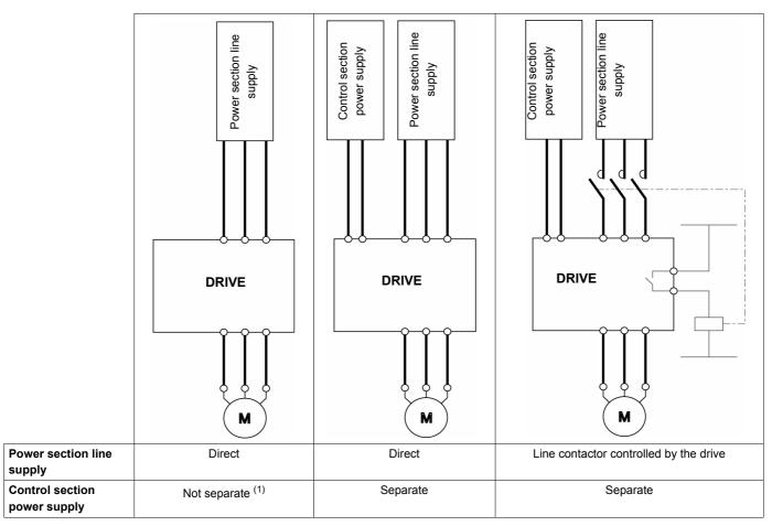
(1) The power section supplies the control section.
