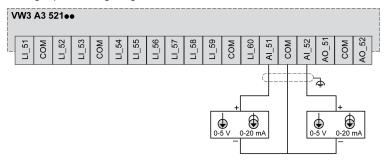
Logic (digital) and Analog outputs wiring diagram:
