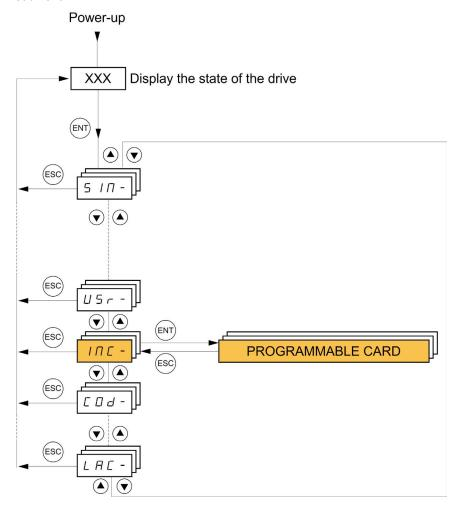
The ATV IMC PROGRAMMABLE CARD menu contains (when not customized) the following submenus:
