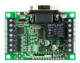
The Wireless 433MHz Receiver provides a fast and simple integration of Security Expert 4 or 2 button remote transmitters into any alarm or access control system. The standalone functionality allows for easy, secure operation of gates or other access areas where convenience is required.
