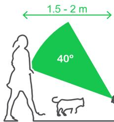
Movement is detected only in the green zone, so small pets won't trigger the light.
