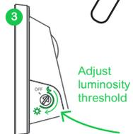
> Wait for the LED to turn OFF ( $\approx 1$ min calibration), set / wait until room illumination is at intended brightness. Adjust daylight setting dial until LED illuminates.
