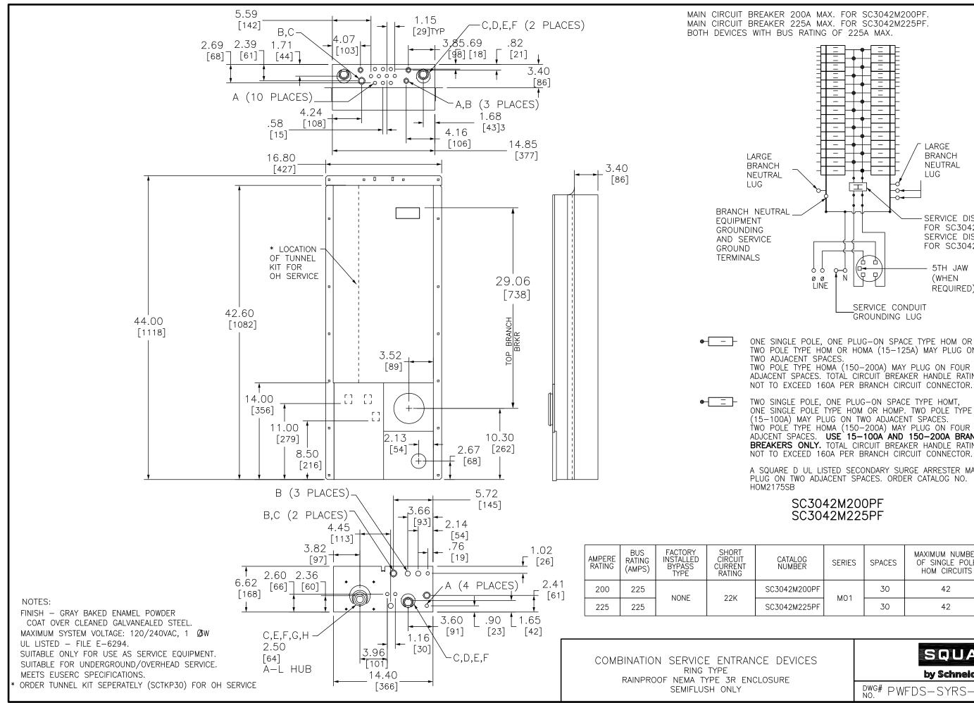
KNOCKOUTS CONDUIT SIZE SYMBOL ММ IN .50 Α 13 В .75 19 С 1.00 25 D 1.25 32 38 Ε 1.50 F 51 2.00 LARGE G 2.25 64 **BRANCH** Н 76 NEUTRAL 3.00 SERVICE DISCONNECT 225A MAX FOR SC3042M225PF SERVICE DISCONNECT 200A Max FOR SC3042M200PF 5TH JAW (WHEN REQUIRED)
