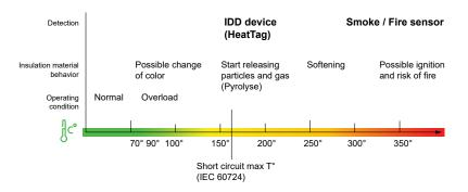
PVC insulation material behavior with increasing temperature
