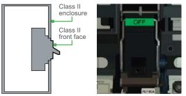
Class II panel with circuit breaker having a class II front face
