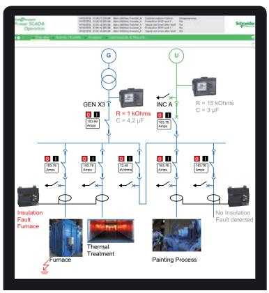
Example of single line diagram including insulation real time monitoring with PSO.
