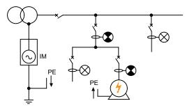
The Insulation Monitor detects and signals an insulation fault based on the alarm threshold set. It activates an alarm relay that can be connected to a sound or light device. It can also send the alarm via communication.
