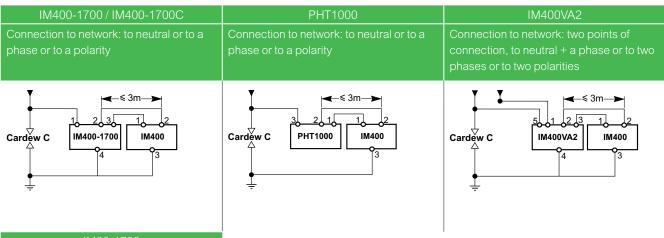
IM20-1700 Connection to network: to neutral or to a phase or to a polarity
