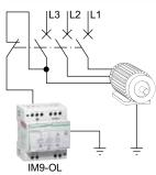
IM9-OL is compatible with any grounding system: IT, TN, TT.
