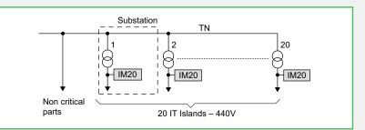
Vigilohm IM20 are monitoring each IT network. Their alarm relay is used to inform the maintenance team of a fault through a light indicator.
