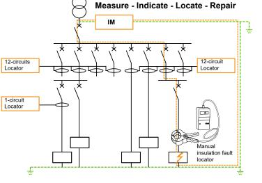
Insulation Fault Locators are associated to an Insulation Monitor. Their measurement principle is based on the low frequency component injected by the Insulation Monitor. Vigilohm range includes permanent Insulation Fault Locators which are connected to the network through toroids (IFL12 range), as well as a manual insulation fault locator kit (XRM and probes).
