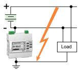
Insulation Monitor injection is wired to one polarity. Whenever the network includes charges or batteries, the injection signal flows over both polarities, allowing to detect an insulation fault affecting any part of the network.
