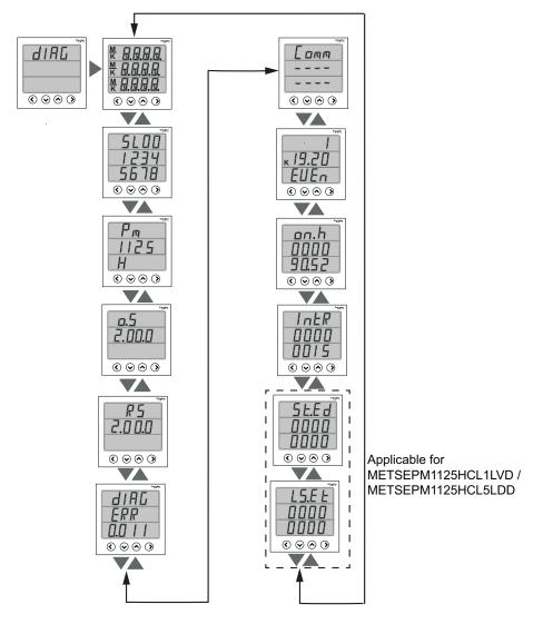
EasyLogic™ PM1125H Display and meter setup
