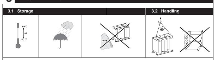
p Use appropriate handling and lifting tools like fork lift, lifting crane for handling for detuned reactor above 25 Kvar or weighing more than 10 kg p During lifting and handling make sure to keep the detuned reactor always in upright position.
