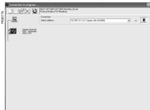
Access to parameters and settings for a Sepam series 60 connected to a communication network.
