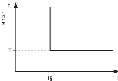
Definite time protection principle.
