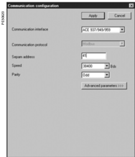
SFT2841: communication configuration window for ACE949.
