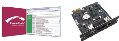
UPS Management PowerChute™ and Network Management Card Remote monitoring and management to allow safe system shutdown for up to 25 servers and workstations
