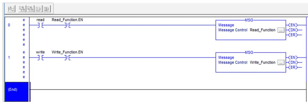
The Read Boolean will trigger the Read\_Function to read the *R C C* parameter.
