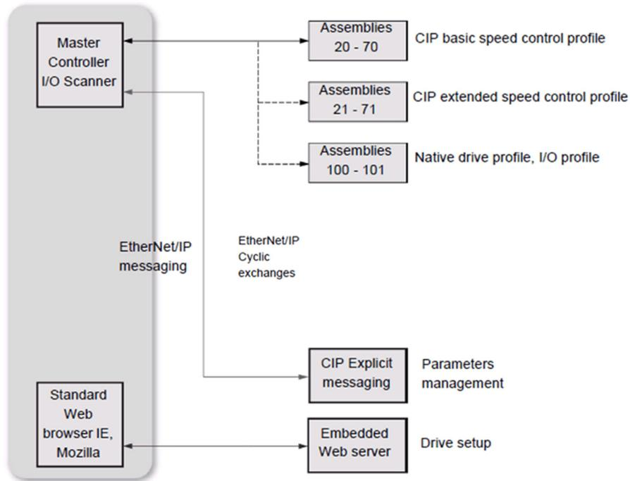
The Ethernet adapter, is compliant with the ODVA drive profile. It supports the following profiles:
