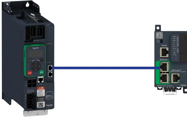
The drive is controlled from the communication but the frequency reference value is adjusted with analog input 1. The control word comes from the controller and is written according to CiA 402 profile.
