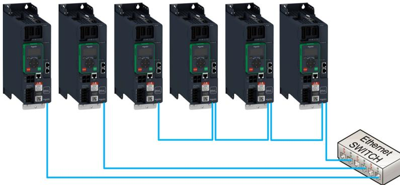
**NOTE:** In daisy chain topology, if one drive is turned off, an **[Embd Eth Com Interrupt] E E H F** error is triggered in the other drives connected to the same topology. To keep the integrity of Ethernet daisy chain network when one or more drives are powered off, add an external permanent 24Vdc supply to the control block of the drive.
