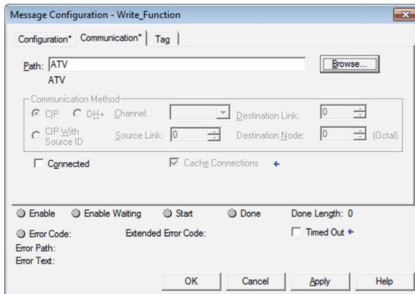
It is possible to read or write the *ACC* parameter by toggling the Read or Write bits.
