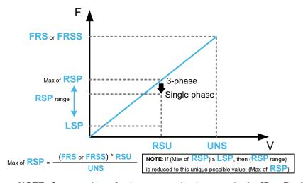
**NOTE:** Compared to a 3–phase power backup supply, the **[Pwr Backup Ref Freq]** RSP value may need to be reduced in order to provide the nominal torque with a single phase power backup supply. For more information, you must refer to the application note "Power Backup".
