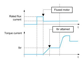
When run command is given, the drive over-fluxes the motor during a short time in order to generate a sufficient motor torque. The level of the torque is set with the parameter [Brk Release Current] IBR. This torque is required to maintain the load during the release of the brake and before starting speed control.
