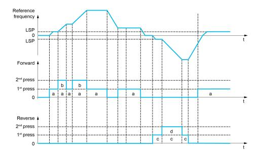
Do not use this +/– speed with double-press buttons with a 3-wire control.
