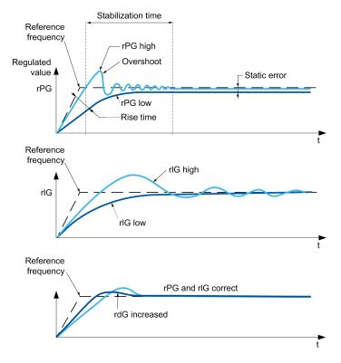
The oscillation frequency depends on the system kinematics:
