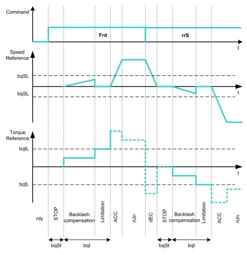
Regulate 0Hz speed at direction change (UC-3)
