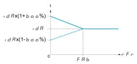
**NOTE:** For synchronous motors, it is recommended to set this value to optimize control at low speed.
