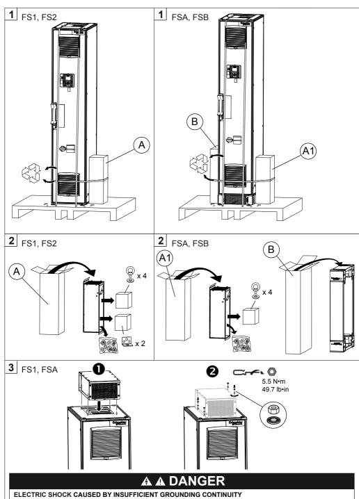
Ensure that all screws, nuts, and washers are properly mounted and tightened as specified in this document.
